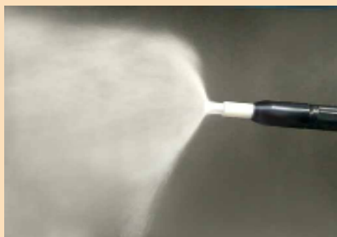
NORMAL GUN WITH EXTERNAL SIEVED POWDER - ALTERED CLOUD PATTERN
