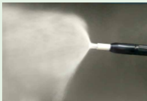
NORMAL GUN WITH EXTERNAL SIEVED POWDER - ALTERED CLOUD PATTERN
